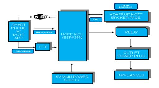
Figure 1. Block Diagram
