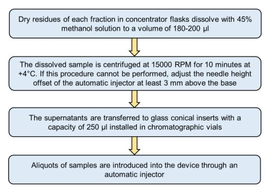
Fig. 5. The procedure steps for performing HPLC/MS analysis
