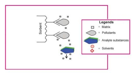
Fig. 3. The process of selective extraction in the cartridge SPE C18, Sep-Pak Plus, Waters
