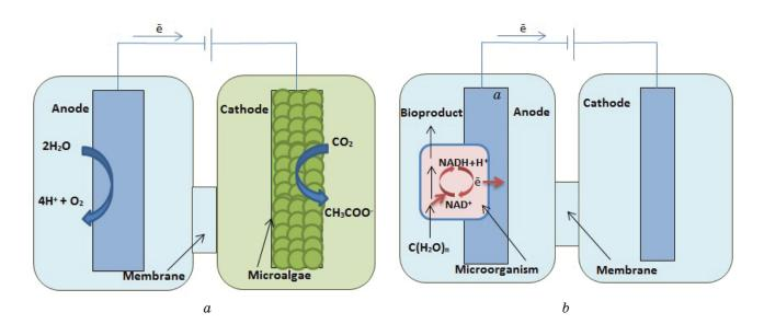
Types of biofuel cells:a — bioelectrochemical control of fermentation; b — microbial electrosynthesis
