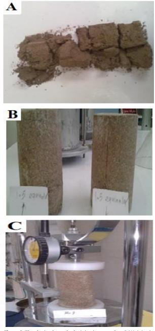
Figure 2: The obtained samples by injection procedure 3 (A), injection procedure 6 (B) and unconfined compressive strength (UCS) apparatus
