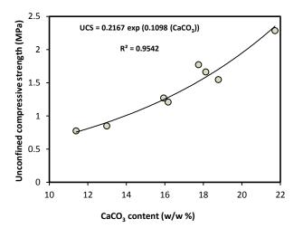
Figure 3: Correlation between unconfined compressive strength and  $\mbox{CaCO}_3$  content
