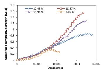
**Figure 4:** Stress-strain curve of biologically treated soil samples at different CaCO<sub>3</sub> contents
