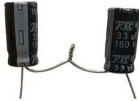
Figure 7. Single-phase AC capacitor. Source: own.
