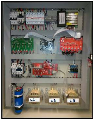
Figure 12. D-STATCOM used for comparison. Source: own.
