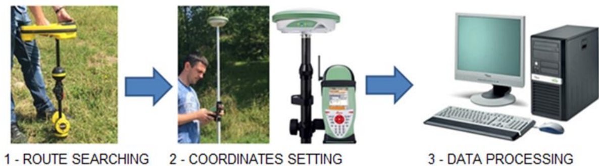
Fig. 3. Procedure for obtaining pipeline SSS data
