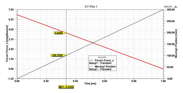
Fig. 7. Variation of acceleration force in time for I=1000A
