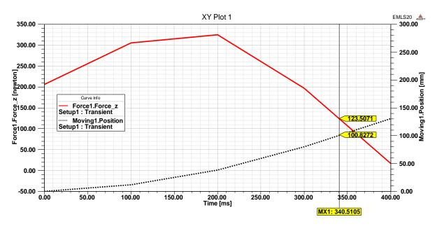
Fig. 5. Variation of acceleration force in time
