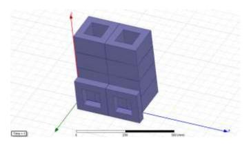
Fig. 2. Moving coils in front of acceleration stages
