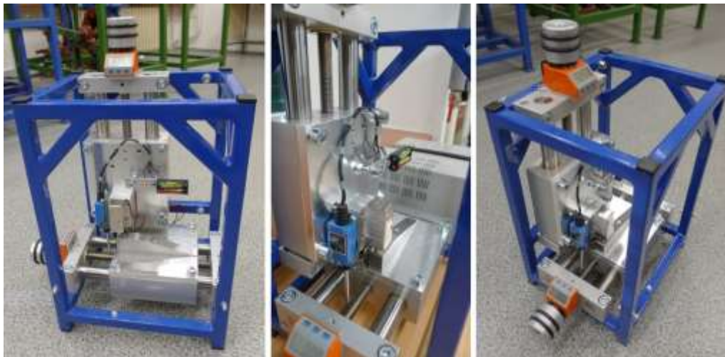
Fig. 3. The constructed test stand site of the innovative pallet locking design
