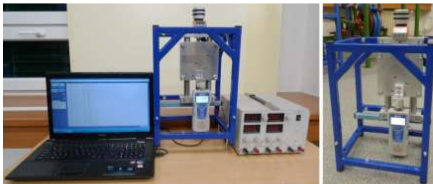
Fig. 7. Constructed measuring station of holding force of the DC electromagnet
