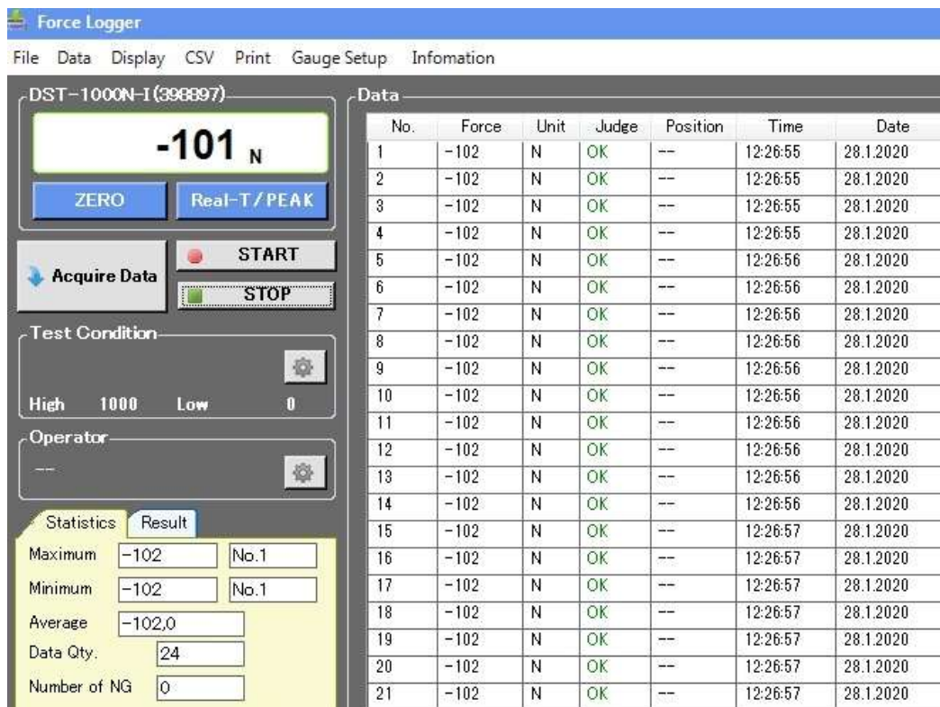
Fig. 5. The holding force of the electromagnet, detected by a digital load cell, was recorded on a PC by the Force Logger software, ver. 1.01
