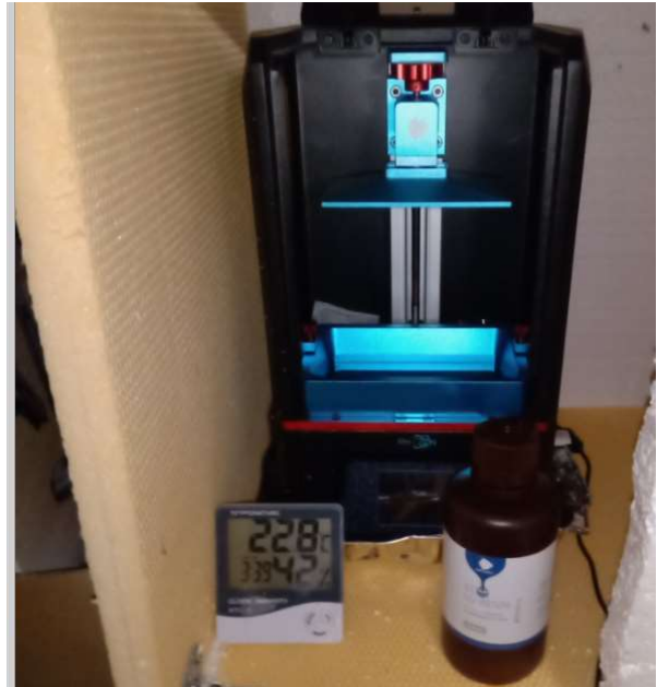
Figure 2. Printer, thermal chamber, apparatus measuring thermal conditions and resin used
