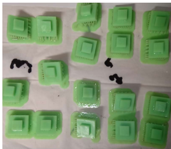
Figure 4. Item printed at different thickness for studying dimensional influence
