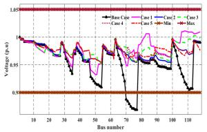
Fig. 14: Bus Voltage Profile of Case I to Case 5 for IEEE119 Bus System
