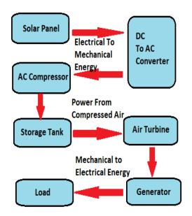
FIG. 4. ENERGY FLOW DIAGRAM
