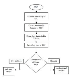
Fig. 4. Flow diagram for key authentication
