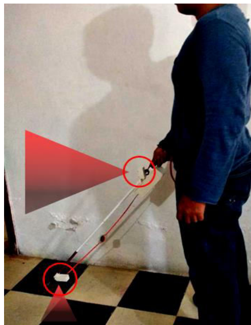
Figure 7. Device functioning. The triangles in red are the area of detection; and the red circles are the ultrasonic sensors.
