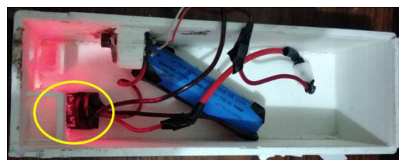
Figure 3. Power bank in the case of the device, Yellow circle is the charging element.
