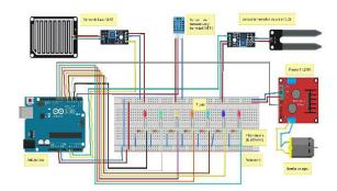
Figure 2. Connection diagram of the autonomous urban garden.
