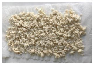
Figure 1. Paper pulp obtained with NaClO2 method
