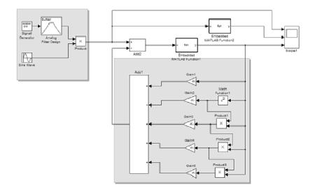
**Figure.2.** Matlab Simulink developed file to simulate the reduction of nonlinearity of radiofrequency stages by introducing a feedback loop based on the reverse power series
