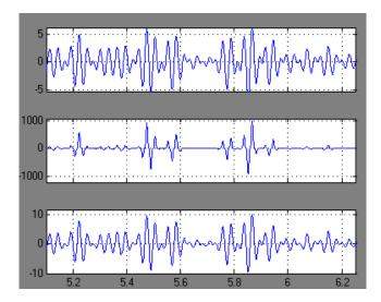
**Figure.3.** The signals obtained from the Matlab-Simulink simulation according to Fig.1: a) the original signal b) the amplified signal without compensating for the nonlinearity c) the amplified signal by feedback loop introduction based on the reverse power series
