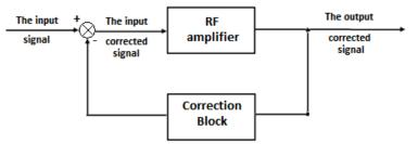
Figure 1. Compensate the operating effects of RF amplifiers in the nonlinear area by introducing a feedback loop
