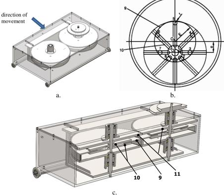
**Figure 3**. Construction of the IPS [20] a. general view; b. arrangement of the balls; c. cross section
