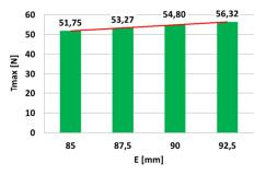
Figure 8. Influence of the radius E on the maximum propulsion force
