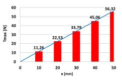
Figure 7. Influence of the eccentricity *e* on the maximum propulsion force
