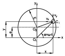
Figure 4. Kinematic of a ball
