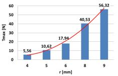
Figure 6. Impact of the ball radius r on the maximum propulsion force
