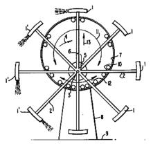
Figure 2. Haller's propulsion apparatus [8]
