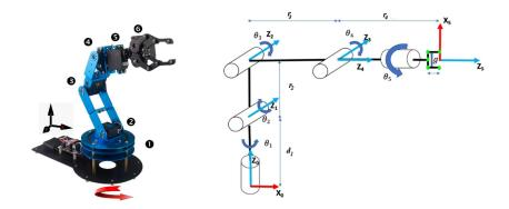
**Figure 1**. D-H Parameters of the testing robot (left – real model; right - virtual 3D model).
