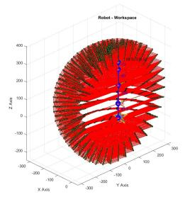
Figure 5. Robot working space in half-representation
