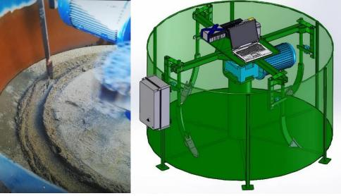
Fig. 1 – Experimental stand for testing chisel knives
