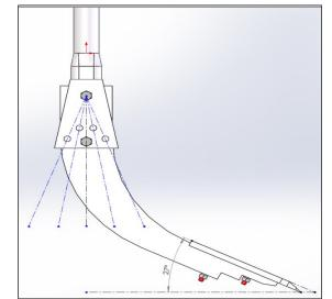
Fig. 4 - Adjusting the angle of attack on the tool holder
