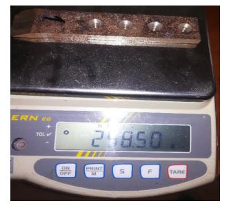
Fig. 5 - Chisel knives weighing
