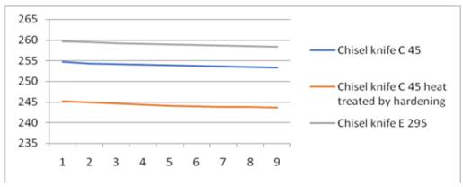
Fig. 6 - Evolution of the wear of the 3 chisel knives
