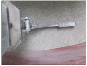
Fig. 3 - Chisel knife mounted on the experimental stand
