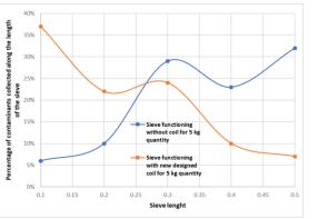
b) The distribution of contaminants collected on the sieve length for a quantity of 5 kg of input material; comparison between the sieve functioning with and without the new designed coil
