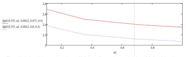
Fig.4 – Variation of the sorted seed mass (Qs) depending on the speed of the coil ( $n_1$ ) and the advance speed of the grains in the helical movement ( $V_M$ )
