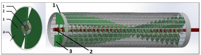
Fig. 6 – Overview of the new proposed subassembly, made of a sieve and a helical coil with the customizable blade angle of attack set to 45 degrees 1 – the sieve having perforations with size 2.24 x 20 mm.; 2 – the axis of the rotating coil; 3 - rotating coil blades;
