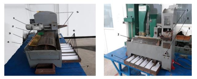
Fig. 1 - Rotary wheat separators pilot experimental stand (1) drive motor, (2) sieve, (3) brushes, (4) axis of rotation, (5) feeding inputs, (6) impurity collection trays, (7) clean wheat tray, (8) start / emergency stop button, (9) hydraulic jack
