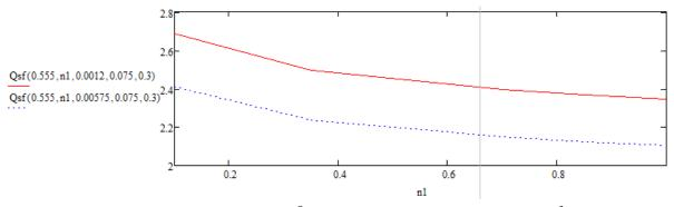
Fig. 5 – Variation of the sorted seed mass (Qs) depending on the speed of the coil (n1) and the distance between the blades of the coil driving grain inside the sieve (De)
