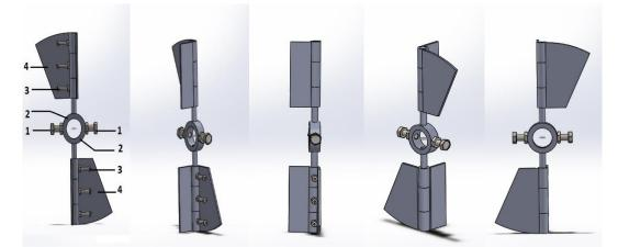
Fig. 8 – The subassembly blades installed on the coil axis, having the role of breaking the immobile nucleus 1– fastening screws for attaching the blade to the coil axis; 2 - bushing; 3 - fastening screws to vary the winding of the coil; 4 – wing blade
