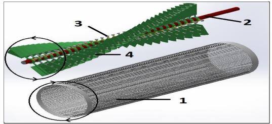
Fig.7 – Driving assembly, designed to run in the opposite direction of the sieve and the coil increasing the agitation level of wheat grains
