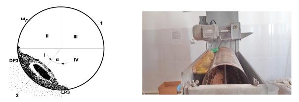
Fig. 3 – Movement of seeds in the layer, inside the sieve Note: modified diagram after Jianbo, Y. et. al., (2018) 1– Cylindrical sieve; 2 - the immobile nucleus; DP3 -detachment point; LP3 - landing point
