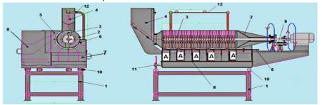
**Fig. 10 - Representation of the newly designed subassembly installation in a cylindrical rotary separator** 1- sieve body; 2- sieve drive module in the opposite direction to the coil; 3 - inner helical coil; 4 - feeding hopper; 5 - support for collection trays; 6 - collection trays shutter; 7 - horizontal collecting chamber; 8 - vertical collecting chambers; 9 - motor drive group; 10 - joint; 11 - sieve angle adjustment screw; 12 - sieve cleaning brush.
