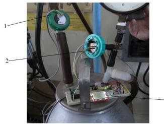
**Fig. 8 – General view of the measurement system of vacuum gage pressure fluctuation** 1 – the sensor vacuum gage pressure of the line type; 2 – the one-port vacuum gage pressure sensor;
