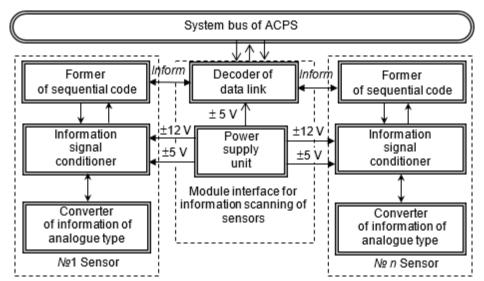
Fig. 2 - The structural chart of the interface for receiving and transmitting the data of ACPS sensors
