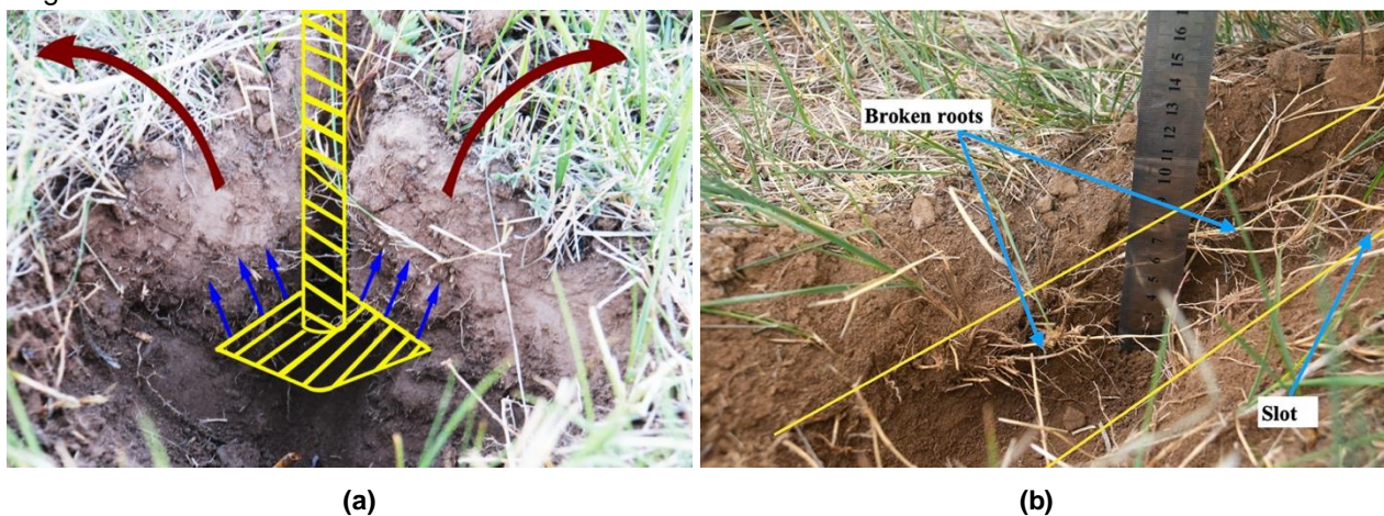
Fig. 5 - Soil disturbance underground: (a) schematic diagram of the coupling failure mechanism between opener and soil layer, (b) broken roots caused by openers
