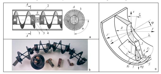
Fig. 1 - Design and calculation scheme of the screw working body, the sections of which are hinged a - the image of two sections; b - is a general view of sections of a working body located on a curved section and its individual elements; c - scheme for determining the forces acting on the elementary volume of bulk material that moves inseparably in the casing
