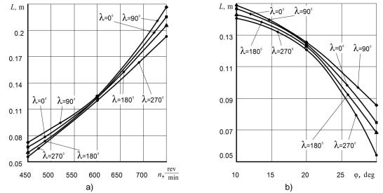
Fig. 2 - Graphical dependences of the free flight range of the material particle L on the rotation speed of the working body n (a) and the angle of inclination of the screw section axis to the horizon (b) at different angular positions  $\lambda$  of the particle at the time of separation from the screw edge to contact with the lower surface of the casing
