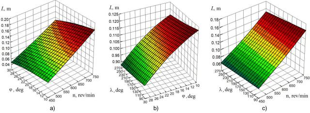
Fig. 3 – Response surfaces of the flight range of the material L: a - L =  $f(\varphi; n)$ ; b - L =  $f(\lambda; \varphi)$ ; c = L =  $f(\lambda; \varphi)$
