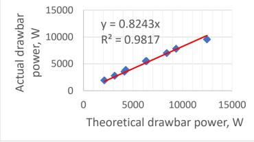
Fig. 4 - Mechanical power loss due to travel reduction ratio
