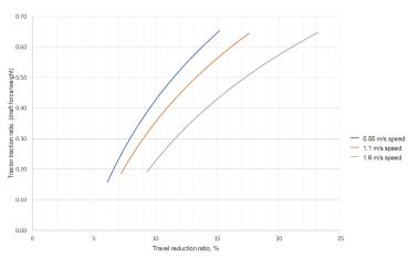
Fig. 3 - Tractor traction ratio versus travel reduction for different theoretical speeds
