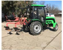
Fig. 1 - Experimental model of electric tractor with plough mounted on
