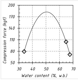
Fig. 10 - Effect of moisture content on compression force
