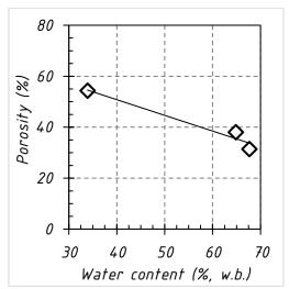
Fig. 8 - Effect of moisture content on porosity
