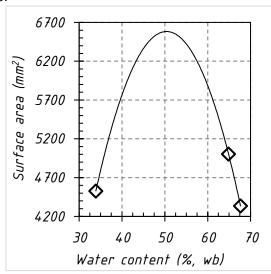
Fig. 5 - Effect of moisture content on surface area
