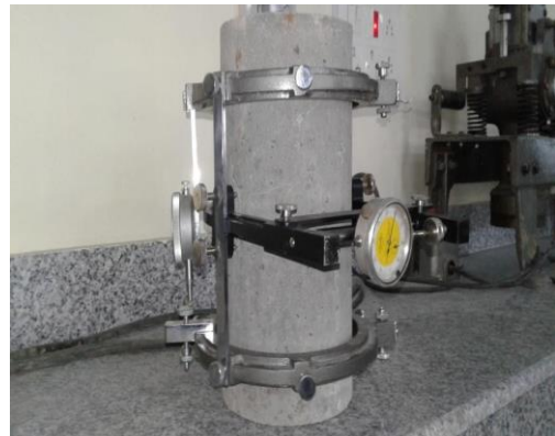
Figure 1. Cylindrical specimen fitted with a compressometer extensometer arrangement
