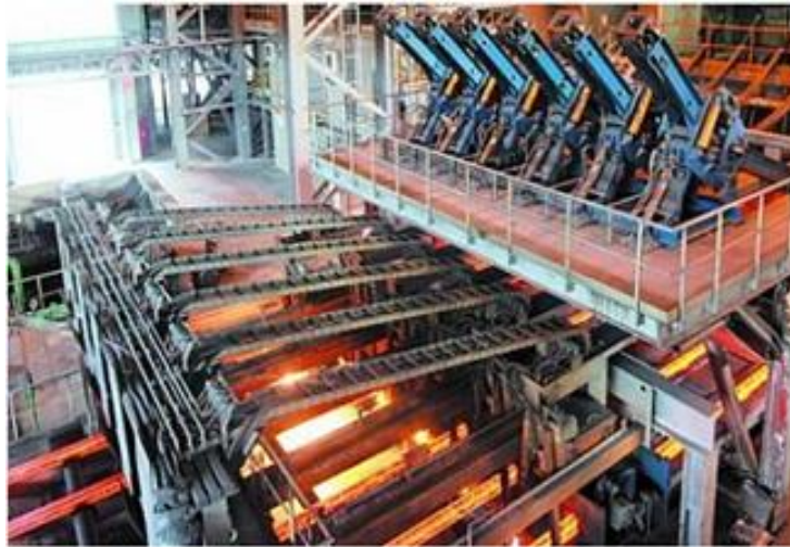
Figure 9. A six-roll continuous casting machine for billets of steel 0.15x0.15 m in size at the converter shop of Public Company «Arselormittal Kryvyi Rih» (Press –release: «Arselormittal Kryvyi Rih», 2011)
