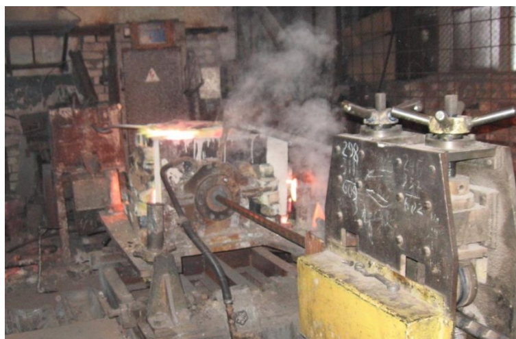
Figure 2. Experimental machine of horizontal continuous casting of copper alloy billets «Energoprom» LLC (Author's photo).
