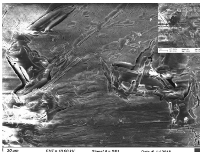
Fig. 12. SEM results of the control MAP crystal and well inhibited (C+5) MAP crystal
