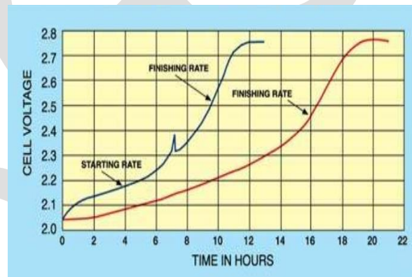
Fig 1.0: Characteristic curve of Plante Cells [1] Fig 2.0: Complete Discharge Characteristic curve of Plante Cells [1]
