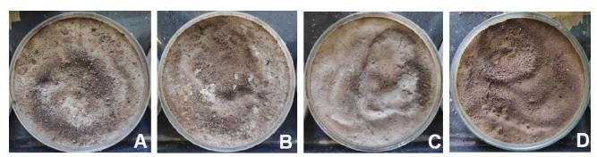
Figure-5 Consolidation block after curing of 21 days by spraying 5ml media/ day showing whitish layer on the block indicate the precipitation. (A) Isolate 1, (B) Isolate 2, (C) Isolate 3 and (D) Control.
