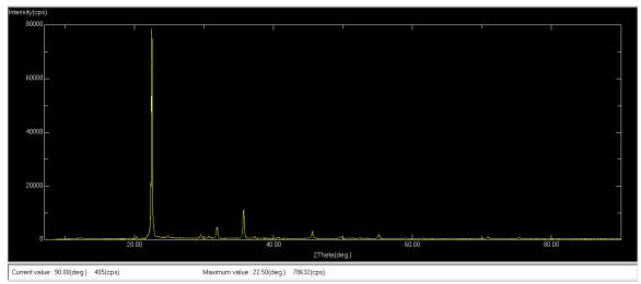
Figure 7: shows X-ray diffraction pattern of crystalline phase present in the production media after the incubation showing the calcite present in the media which is precipitate by the *Bacillus pacificus* MCCC 1A06182.
