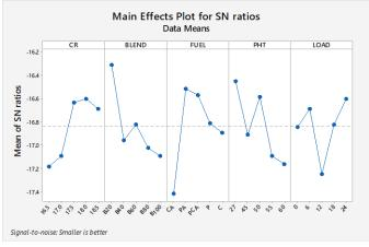
Fig.6: SN Ratio for Brake Thermal Efficiency
