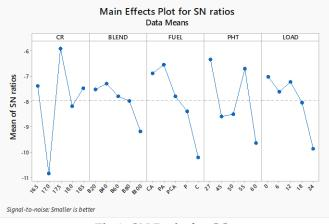
**Fig.2: SN Ratio for CO**<sub>2</sub> Optimal combination for CO<sub>2</sub>: 17.5/B40/PA/27/0
