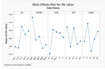
Fig. 5: SN Ratio for Brake Specific Energy Consumption Optimal combination for BSFC: 17.5/B20/PA/27/6
