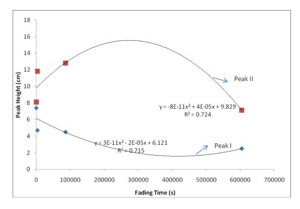
Fig. 6: Fading pattern of synthetic fused quartz with <sup>60</sup>Co irradiation source
