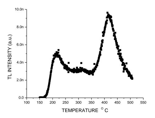
Fig.4: Glow curve of synthetic Fused quartz with 5 °C/s cycle time and 150 °C preheat using <sup>90</sup>Sr/<sup>90</sup>Y source with irradiation for 1 h
