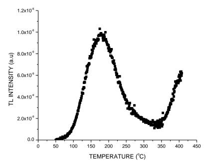
Fig.1: Glow curve of synthetic Fused quartz with 5 °C/s heating rate using 6°Co with irradiation for 1h
