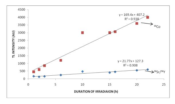
Fig. 5: Dose response of synthetic Fused quartz with <sup>60</sup>Co and <sup>90</sup>Sr/<sup>90</sup>Y irradiation sources respectively
