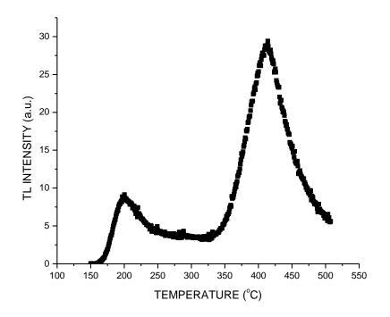
Fig. 3: Glow curve of synthetic Fused quartz with 5 °C/s heating rate and 150 °C preheat using <sup>60</sup>Co source with irradiation for 1 h
