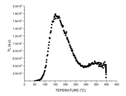
Fig. 2: Glow curve of synthetic Fused quartz with 5 °C/s heating rate using 90Sr/90Y source with irradiation for 1 h
