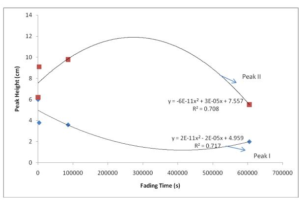
Fig. 7: Fading pattern of synthetic fused quartz with <sup>90</sup>Sr/<sup>90</sup>Y irradiation source
