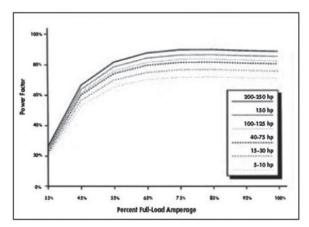
FIGURE 2: Motor power factor (as a function of the % full-load amp) [4]
