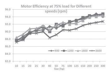
FIGURE 5: Motor efficiency at 75% load.
