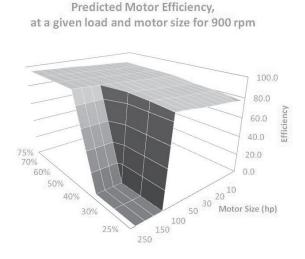
FIG 12: PREDICTED MOTOR EFFICIENCY, KNOWN LOAD AND MOTOR SIZE AT 900 RPM
