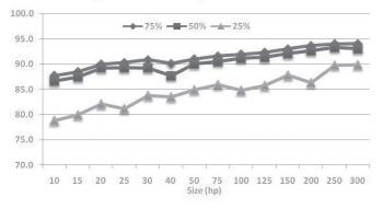
FIGURE 4: average motor efficiency for different rated loads.
