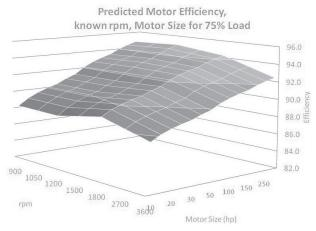
Fig 8: Predicted motor efficiency, at a given rpm and motor size, at 75% load
