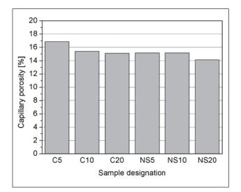
Fig. 8. Capillary porosity of cement mortars
