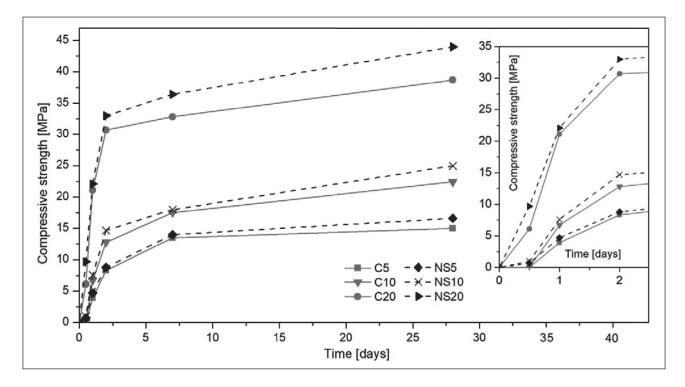
Fig. 2. Compressive strength of mortars after 12 h and 1, 2, 7, 28 days of curing
