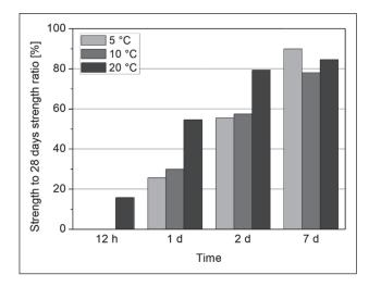
Fig. 4. Compressive strength to strength for 28 days ratio, control samples
