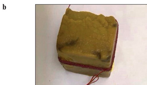
Fig. 1. Cement stone samples after acid corrosion: a – the content of calcium polysulfide – 3%; b – the content of calcium polysulfide – 5%
