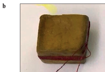
Fig. 2. Cement stone samples boiled after acid corrosion: a – the content of calcium polysulfide – 3%; b – the content of calcium polysulfide – 5%
