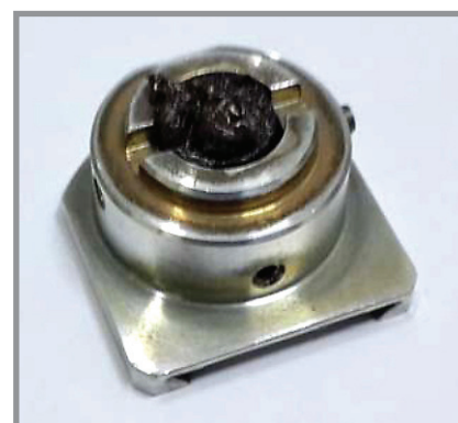
Fig. 3. Binder sample after SEM coating
