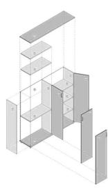
Figure 1. A detailed picture of the constructive parts of the window-case
