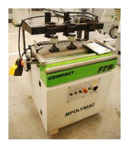
Figure 4. Traditional drilling machine F21N COMPACT
