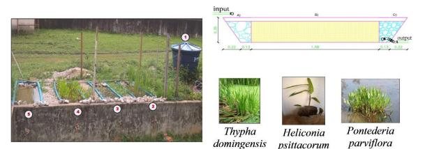
1Reservoir; 2 CW planted with Thypha; 3 CW planted with Heliconia; 4 CW with Pontederia; and 5 CW not planted. A) stone hand; B) sand; C) gravel  $N^{\circ}$  2
