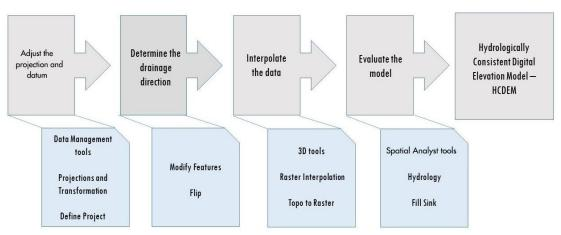
**Figure 2.** Procedures employed for determining the Hydrologically Consistent Digital Elevation Model (HCDEM).
