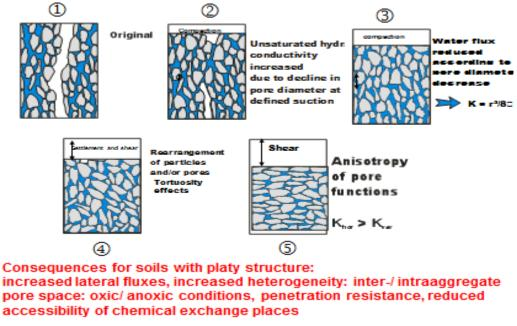
Figure 7. Stress and strain effects on hydraulic properties
