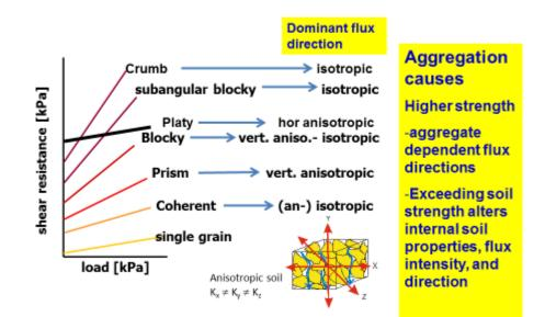
**Figure 4.** Aggregate dependent pattern of the Mohr Coulomb failure lines and associated dominant flux directions.
