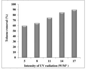
**Fig. 4:** Effect of UV Lamp intensity on toluene removal efficiency (300ppm toluene concentration - 45% relative humidity)
