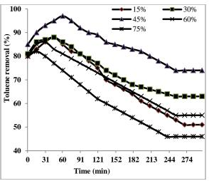
Fig. 6: Effect of relative humidity on toluene removal efficiency (toluene concentration of 300 ppm and UV intensity of  $17 \text{ w/m}^2$ )
