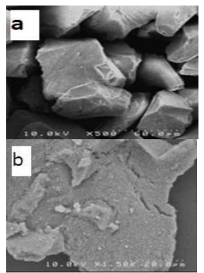
Fig. 2: Micrograph prepared by a scanning electron microscope from the silica gel bed (a) and catalyst  $TiO_2/SiO_2$  (b)
