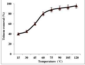
Fig. 5: Effect of reactor column temperature on toluene removal efficiency (300 ppm toluene concentration - relative humidity 45% - intensity of UV radiation 17 w /  $m^2$ )
