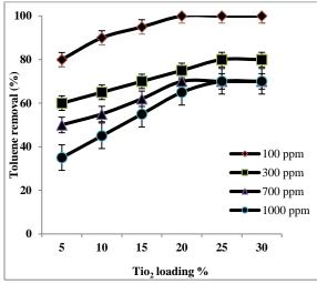
Fig. 3: Toluene photocatalytic oxidation efficiency using  $TiO_2$  /  $SiO_2$  catalyst (catalyst; 5 to 30 wt.%, toluene concentration; 100 to 1000 ppm, apparent gas velocity; 2 l/m, humidity; 45%).
