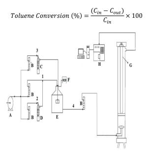
**Fig. 1**: Schematic diagram of the fluid bed reactor along with a system for providing the pollutant-specific concentration and relative humidity. Air Blower (A), Rotameter (B), Water Impinger (C), Toluene Impinger (D), Mixing Enclosure (E), Moisture Sensor (F), Fluid Bed Reactor (G), Gas Chromatography (H)
