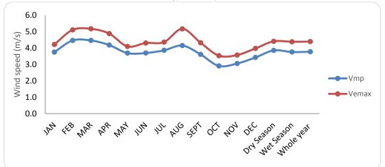
Figure 11: Plot showing the variation of the most probable wind speed (Vmp) and the wind speed carrying maximum energy (Vemax) for Ijebu-ode.
