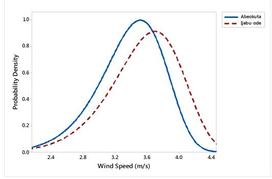
Figure 4: Probability Density Function for Whole Years at Height of 10m
