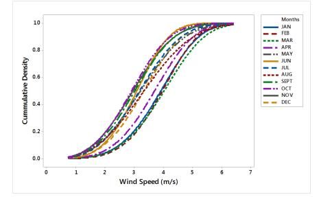
Figure 7: Cumulative Distribution Function for whole years at Height of 10m for Abeokuta.
