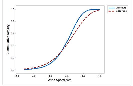
Figure 5: Cumulative Distribution Function for whole years at Height of 10m
