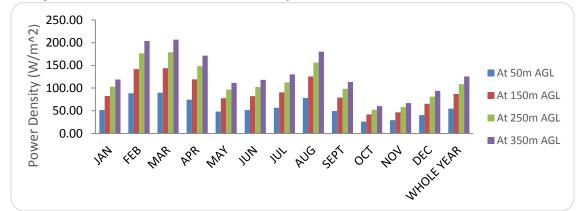
Figure 13: Plot showing the monthly variation of Power densities for the extrapolated means Wind speeds for Ijebu-Ode
