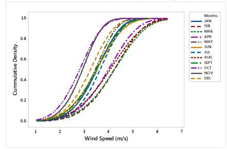
Figure 8: Cumulative Density Function for Whole Years at Height of 10m for Ijebu-ode
