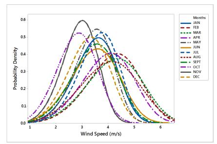
Figure 9: Probability Density Function for Whole Years at Height of 10m for Ijebu-ode
