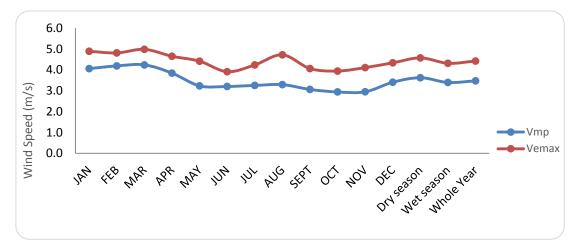
Figure 10: Plot showing the variation of the most probable wind speed (Vmp) and the wind speed carrying maximum energy (Vemax) for Abeokuta.
