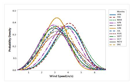
Figure 6: Probability Density Function for Whole Years at Height of 10m for Abeokuta.
