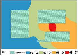
**Figure 3:** Measurement stations and the arrangement of machinery in the compressor unit (A), noise map of the compressor unit with different zones of SPL interval (B)
