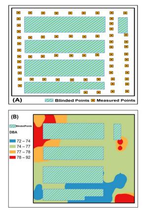
**Figure 2:** Arrangement of boilers and measurement stations in the boiler hall (A), noise map of the boiler hall (B)
