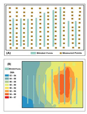
Figure 1: Arrangement of machinery in the spinning hall, with the horizontal positions of the measurement stations, and blinded
