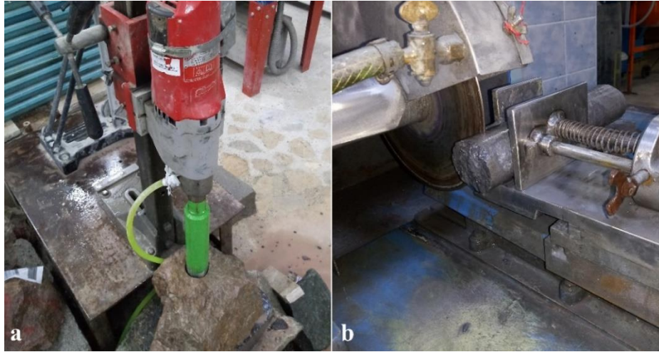
Figure 1: a) Rock coring, b) core cutting by using sawing machine
