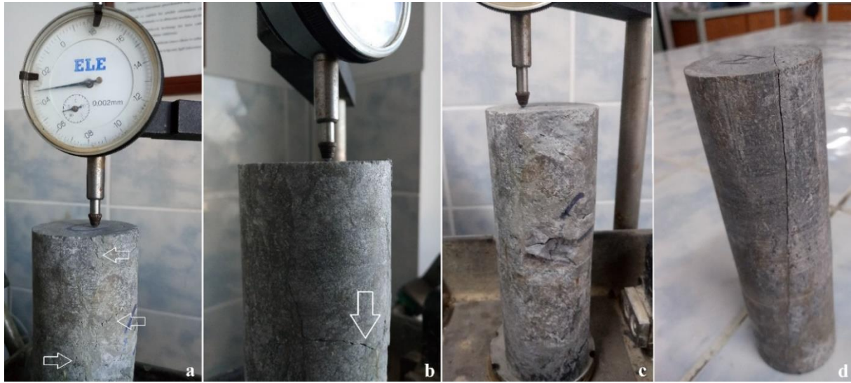
Figure 7: Some crack shapes observed from this study: a) Narrow cracks, b) a major cracking, c) disintegration, d) disintegration by a long crack all through the specimen
