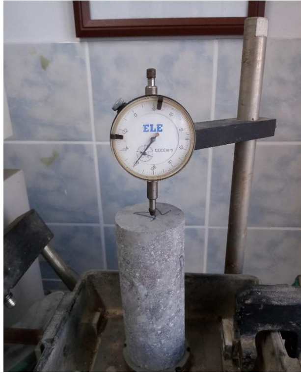
Figure 5: Cooling strain measurement using dial gauge
