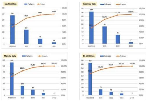
Figure 4. Total number of failures by type line production (July 2018)
