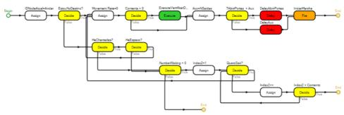
Figure 2. Process responsible for deciding an elevator stop
