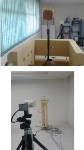
Figure. 22 Photograph of the proposed antenna during the measure of the gain
