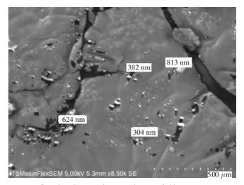
Figure 1. Scanning electron microscope images of chitosan-*Pinus merkusii* extract nanoparticles showed irregular shape, and the morphology surface showed the rough surface.
