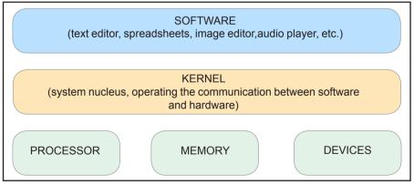
Note: Kernel is the center of an operating system, its nucleus. It is responsible for serving as a bridge between the software and the hardware of a computer. Front-End users (interface-users) are generally limited to the knowledge of the software, without the need to understand the inner workings of the computer at the other levels. We can make an allusion to the visible part of an iceberg, when the major part of the rock is submerged and outside of our field of vision.
