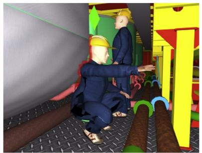
Figure 2. Ergonomic check of the design using dummies (Source: [1]).
