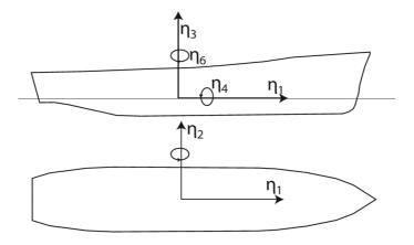
Figure 3. Ship coordinate system (Source: [5]).
